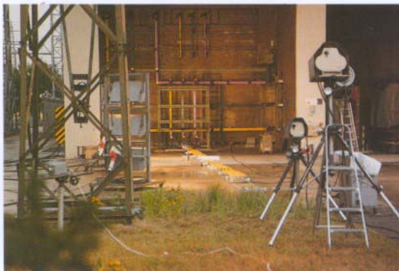
Conductor rail system tested for short-circuit strength at the research institute of high voltage and high amperage technology in Mannheim. Test procedure shot with a high-speed camera (3000 pictures/sec.).
