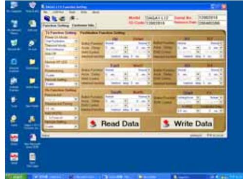
2-4. After changing the function setting (refer to Appendix I & II), either to save the setting data to computer hard disk or write it to another transmitter or receiver. To save the data, click “Save File”, after destination chosen and file name typed, click “Save”. Click “OK”
