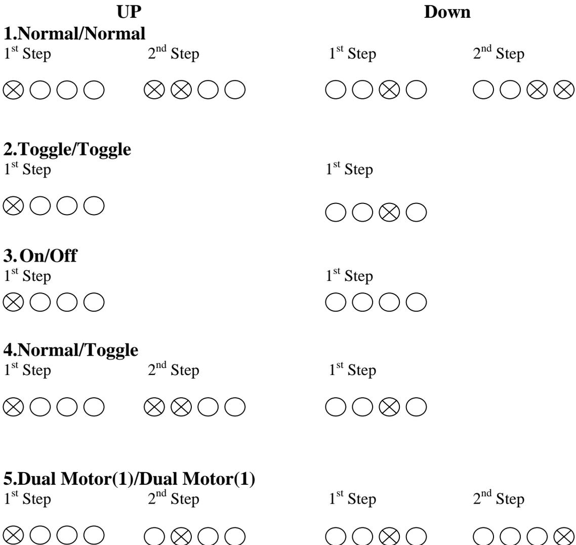
Note: When pushbutton is released from 2<sup>nd</sup> speed and back to 1<sup>st</sup> one, the 1<sup>st</sup> speed relay is activated again till the pushbutton is totally released.
