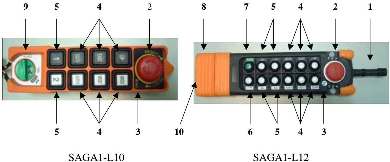
Figure 4-1 Transmitter Configuration
