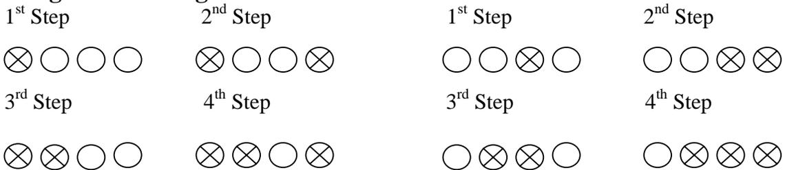
Note: The second step pushbutton must be pressed and held when pushing or turning “Start” pushbutton or key to reach the third and fourth speed.
