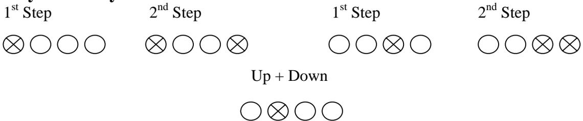
Note: When Up and Down pushbuttons are pressed at the same time the second relay works as “Toggle”, released when they are pressed simultaneously again.
