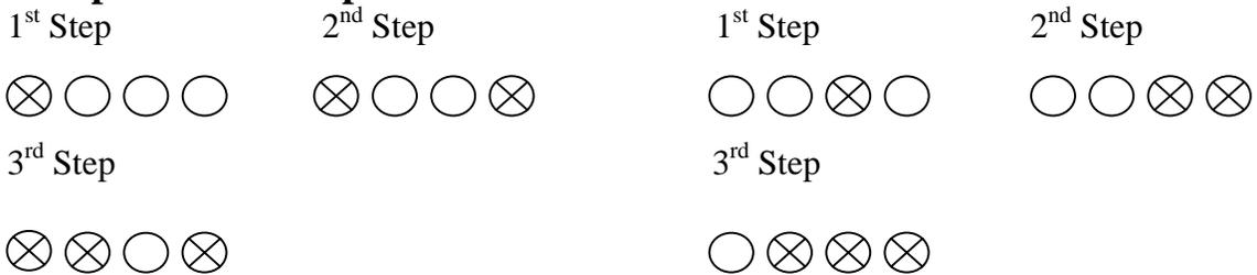
Note: The second step pushbutton must be pressed and held when pushing or turning “Start” pushbutton or key to reach third speed.
